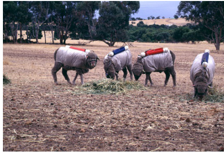
Testing Australian sheep for exhaled methane production (2001), CSIRO
